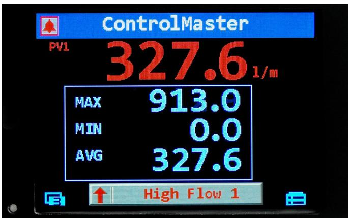
Fig. 2: Single PV indication template display
