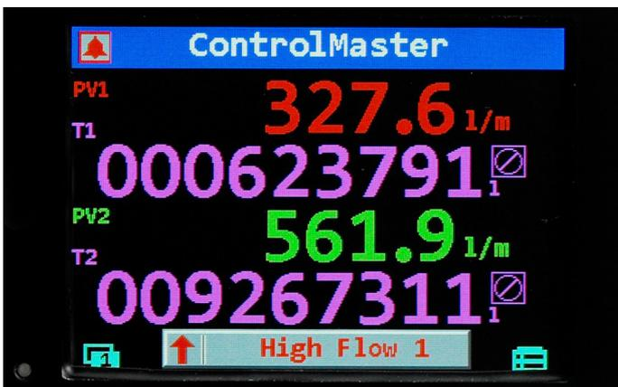
Fig. 3: Dual PV and totalization display
